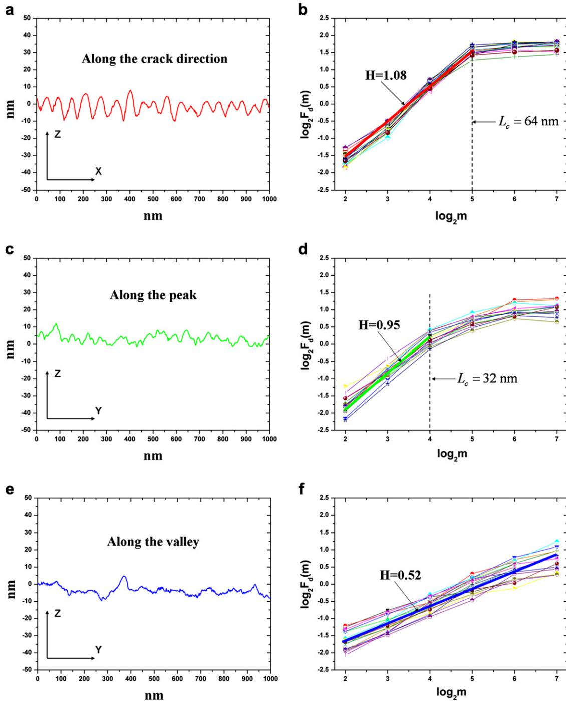
**Fig. 2.** Representative AFM profiles (left column) and their corresponding DFA results (right column) of NPC (a)–(b) along the crack direction, e.g. the red line in Fig. 1b, (c)–(d) along the peak, e.g. the green line in Fig. 1(b) and (e)–(f) along the valley, e.g. the blue line in Fig. 1b. [For interpretation of the references to color in this figure legend, the reader is referred to the web version of this article].
