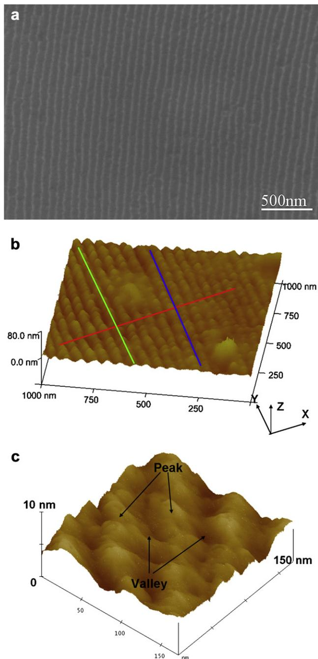
**Fig. 1.** Nanoscale periodic corrugation (NPC) observed on dynamic fracture surface of Vit 1 bulk MGs under high-velocity impact. (a) HRSEM image of the NPC. (b) and (c) AFM 3D image of a NPC at different magnification. [For interpretation of the references to color in this figure legend, the reader is referred to the web version of this article].
