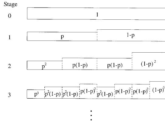
Figure 3. A schematic showing the weights at the first several stages of the binomial multiplicative process.
