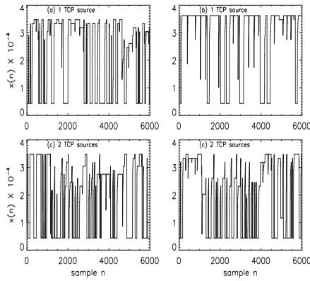
Fig. 2. Time series for the congestion window-size (in Bytes) measured on the Internet.  $w(n)$  has been scaled by  $10^4$ .
