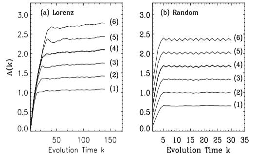
Fig. 1.  $\Lambda(k)$  curves for (a) the chaotic Lorenz attractor with  $m = 4$ ,  $L = 3$  and sampling time 0.03, and (b) a random process with  $m = 6$ ,  $L = 1$ . Curves numbered 1,  $\dots$ , 6 correspond to shells with sizes  $(2^{-(i+1)/2}, 2^{-i/2})$ ,  $i = 5, 6, \dots, 10$ .
