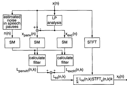
Fig. 1 Block diagram of filtering approach
