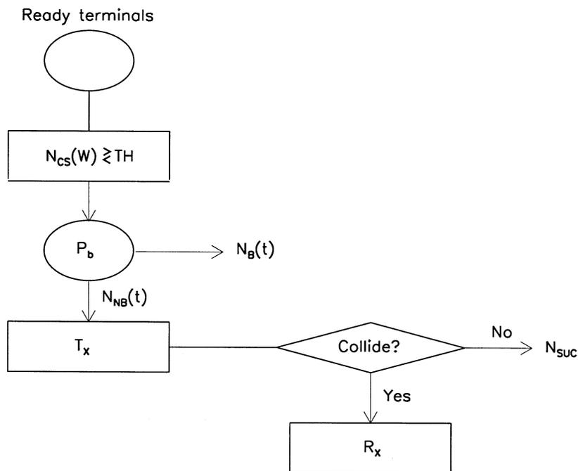
Fig. 1. Schematic of the random-access scheme.
