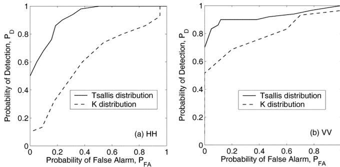
Fig. 4. Receiver operation characteristic curves of the parameter  $\beta$  from the Tsallis distribution (solid lines) and of the parameter  $\nu$  from the K distribution (dash lines) for detecting target among (a) HH and (b) VV datasets.
