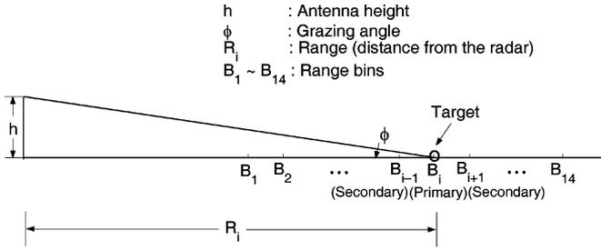
Fig. 1. Schematic showing how the sea clutter data were collected.
