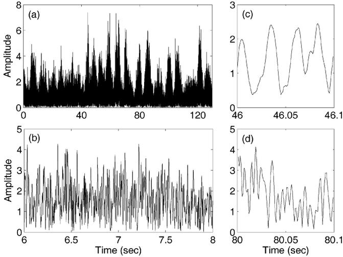
Fig. 2. Example of the sea clutter amplitude data. (a) Entire data, (b) a 2-s segment, and (c, d) two 0.1-s segments extracted from the data.
