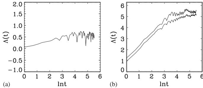
Fig. 2. (a)  $\Lambda(t)$  vs.  $t$  curves for time series generated from the noise-free Henon map with  $a_c = 1.38637288\dots$ ,  $b = 0.01$ . Plotted in (b) are two  $\Lambda(t)$  vs.  $\ln t$  curves (corresponding to two different shells) for the noisy map with  $\sigma = 0.001$ . Similar results were obtained with  $\sigma = 0.0001$ . In the computation,  $10^4$  points were used with embedding parameters  $m = 4, L = 1$ .
