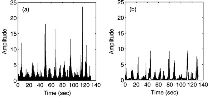
Fig. 1. Examples of the sea clutter amplitude data (a) without and (b) with target. (a) and (b) are plotted using range bin 1 and 9, HH polarization of data file 17 downloaded from the link given in Section II. The radial distance for the data plotted in (a) and (b) is 2574 m and 2694 m, respectively. The azimuth angle for both (a) and (b) is about  $129^\circ$ . Similar figures were shown in [27], [28].
