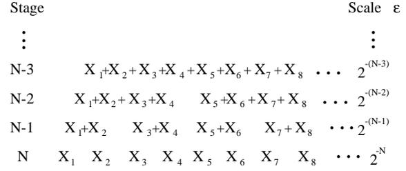
Fig. 8. Schematic for obtaining weights from a time series.
