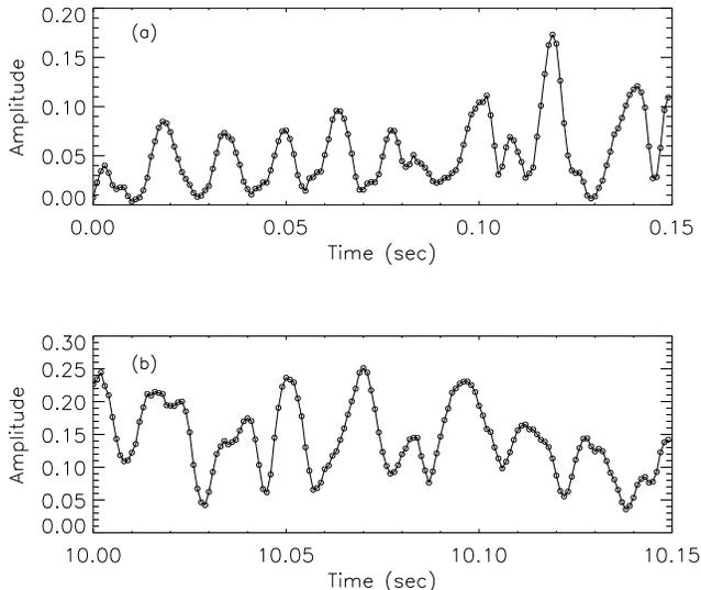
Fig. 1. Two short segments of the amplitude signal of the sea clutter data.
