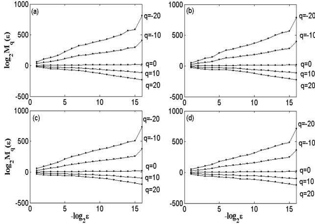
Fig.4  $\log M_q(\epsilon)$  vs.  $\log \epsilon$  curves of sea clutter amplitude data in the same measurement. (a) HH data with primary target; (b) VV data with primary target; (c) HH data without target; (d) VV data without target.
