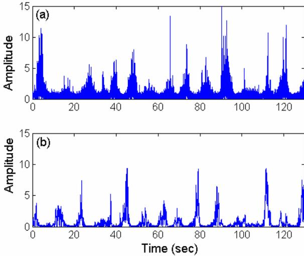
Fig.1 Sea clutter amplitude data from the same dataset. (a) range bin without target, (b) range bin with primary target
