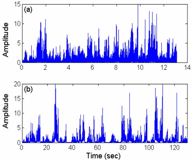
Fig.3 Simulated time series using multiplicative process. (a, b) Simulating sea clutter data in Fig. 1(a, b) respectively.
